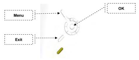
Press the "Exit" button to bring up the Mode Menu. The options in the Mode Menu are: Favorite, Photo, Clock, and Setup. To escape the Mode Menu, press "Exit" again to return to your pictures.
